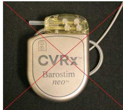
**Incorrect Placement of Lead Behind IPG**
