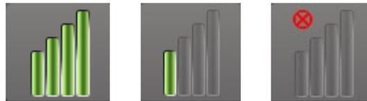
**Figure 9: Link Quality Indicator (Excellent, Poor, No Link)**
