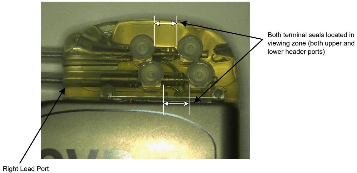
**Figure 18: Terminal Insertion into IPG Header (Correct Insertion)**
