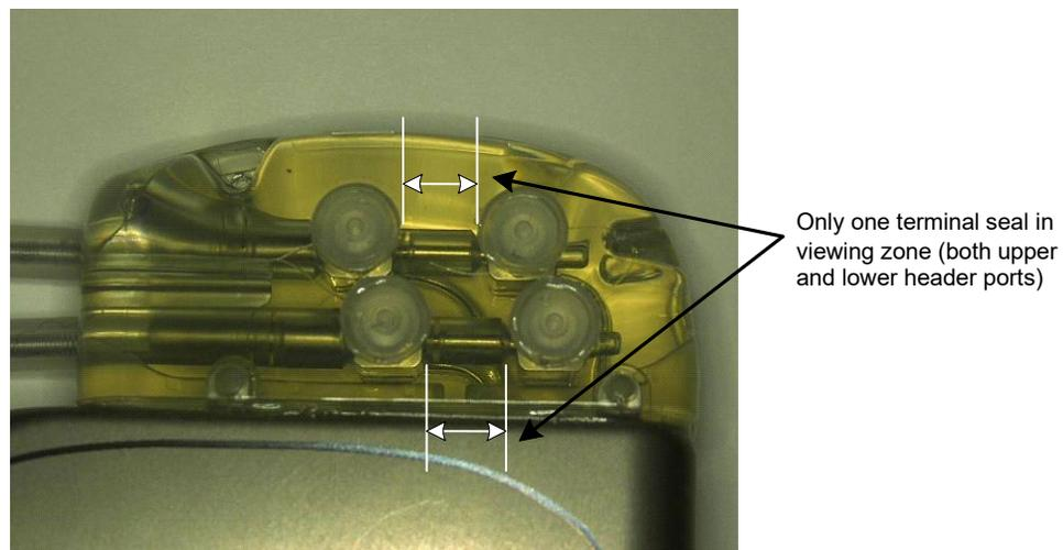
**Figure 19: Terminal Insertion into IPG Header (Incorrect Insertion)**
