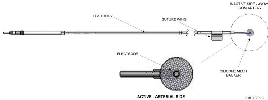
**Figure 3: Carotid Sinus Lead**
