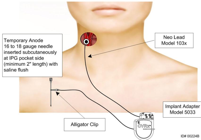
**Figure 11: System Mapping Configuration with Implant Adapter Model 5033**
