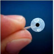
2 mm electrode 7mm silicone backer Unipolar design
