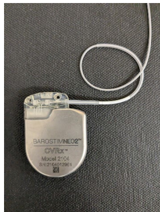
Correct lead body placement
